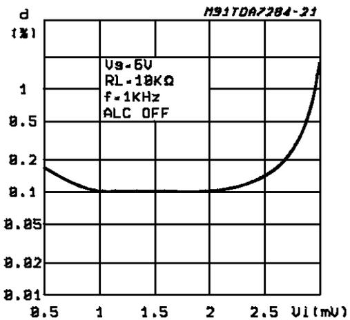
Figure 11: Distortion vs. Input Voltage
