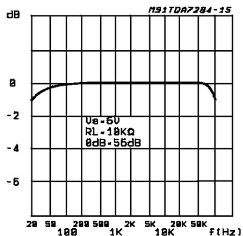
Figure 5: Playback Closed Loop Gain vs Frequency
