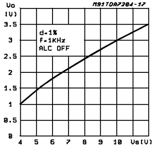
Figure 8: Output Voltage vs. Input Voltage
