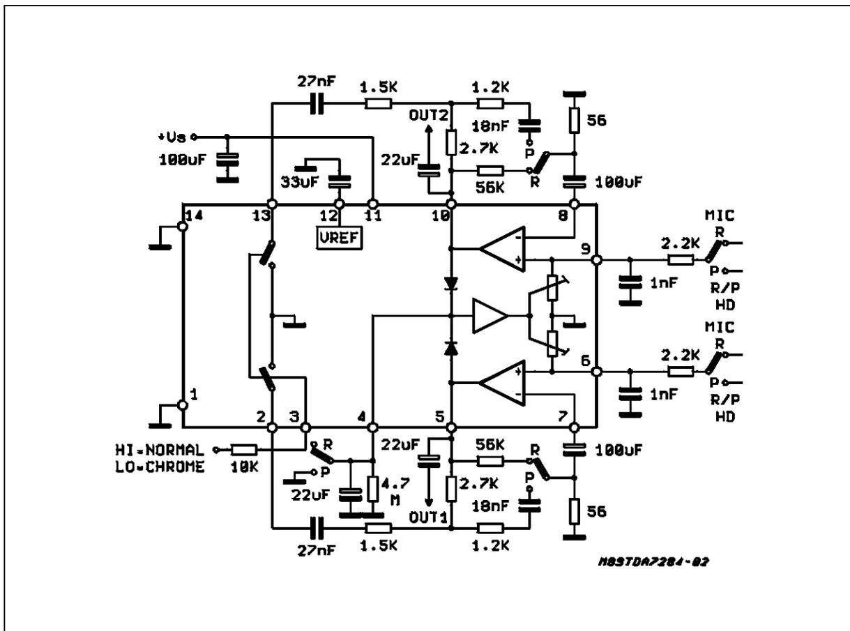
Figure 22: Application Circuit with Output Muting
