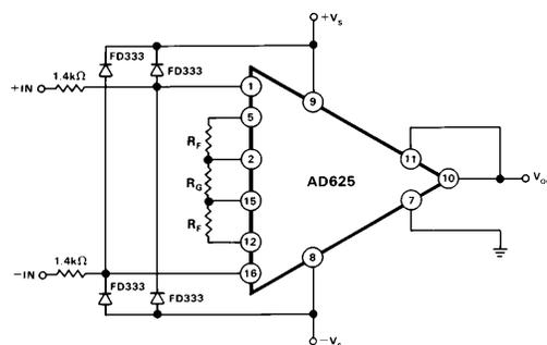
Figure 26a. Input Protection Circuit
