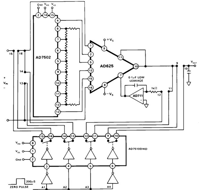
Figure 36. Auto-Zero Circuit
