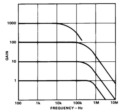
Figure 6. Gain vs. Frequency
