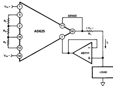
Figure 31. Voltage-to-Current Converter
