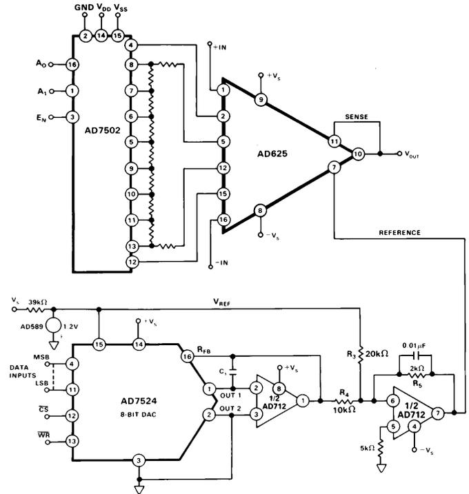
Figure 30. Software Controllable Offset
